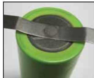
Figure 5. Lithium ion battery with 0.012 inch thick nickel plated copper tab welded to aluminum terminal at 4"/s.
