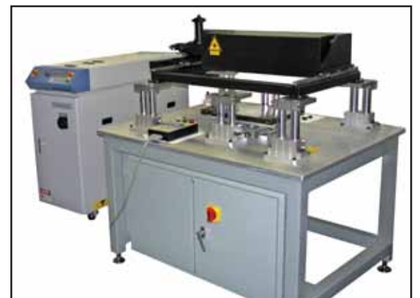
Figure 6. XY gantry laser based solution for battery pack welding, where the pack remains stationary and the focus head is moved.
